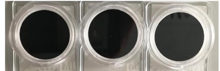
Thermogravimetric analysis of filters indicated  $\sim 95\%$  non-volatile and non-oxidizable material
