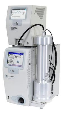
Scanning Mobility Particle Sizer 10-800nm
