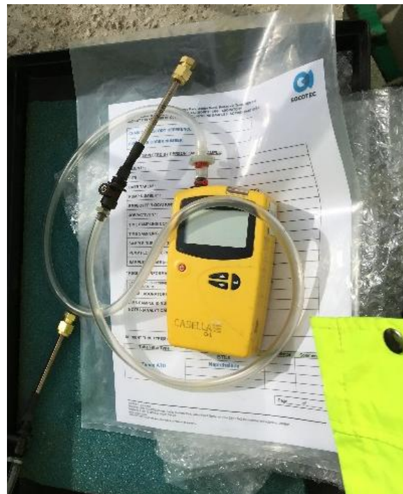
Photo 4.2 – Pumped (active) sampling using a Tenax tube. (Check battery life before going onto site and ensure flow regulator is provided.)
